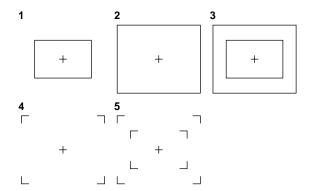
The inner frame and the outer frame are approximately 90% and 95%, respectively, of the safety zone.
